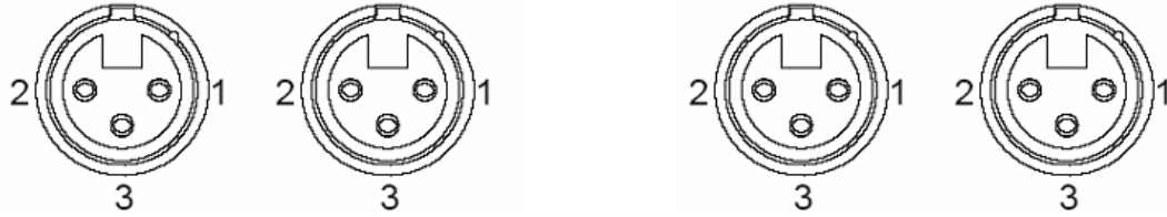
XLR 3p Female-panel Pinout
