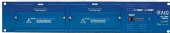
Redundant power supply for AEQ FORUM
