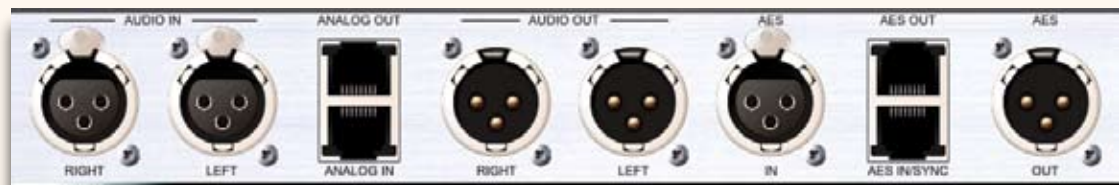
Router Selector Node Rear Panel – Both XLR and RJ-45 connectors are present for inputs and outputs.
