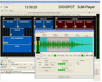
DIGISPOT® has been the first of such systems providing a compliant exchange of the Cart-Wall filled with NAB-cartridges by direct access at a PC video monitor. It became well known under the name CartAssist. Based on the success and the Experiences made with CartAssist the user required the next step to be developed, a Smart Jingle Machine SJM which is now available as a new Module in DIGISPOT®II with extended opportunities to produce a smooth, musically ON-AIR performance.
