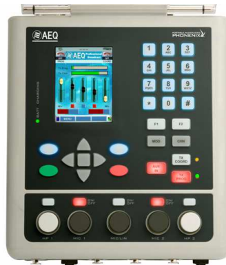
Detail of the Phoenix Mobile control surface and on-screen vu-meters
