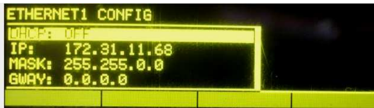
Detail of the configuration of IP address of AEQ Phoenix Studio
