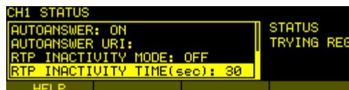
Figure 6: RTP Inactivity detection configuration
